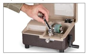
5. To set the diamond tool for a light cut, turn the cut depth adjustment knob clockwise approximately ½ turn after the diamond tool contacts the wheel. If the wheels are of different diameters, use the larger of the two diameters. If necessary, traverse the diamond tool to the left so it does not contact the wheels.
