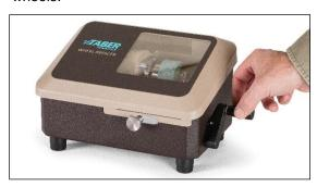
8. Turn the cut depth knob clockwise approximately ½ turn, then continue refacing until the wheel surfaces have been completely renewed. Repeat if necessary.
