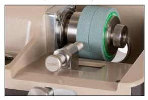
After completing the refacing operation, ensure the diamond tool is returned to the start position (left). Remove the wheels from the wheel arbor and reconnect the vacuum hose to Taber Abraser.
