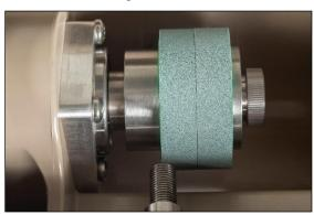
4. Turn the cut depth adjustment knob counter-clockwise until it stops. Then, adjust the diamond tool until the diamond point is approximately 1 mm from the wheel surface. Using the 16 mm wrench, tighten the lock nut to secure the diamond tool in position. This step is only required for initial set-up, and should be completed with a new pair of wheels.
